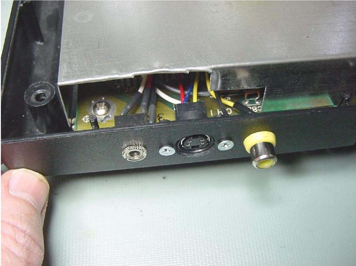
Place the covers back on the power and reset switches, then place the top cover back on. Re-install the 8 screws and lightly tighten.
