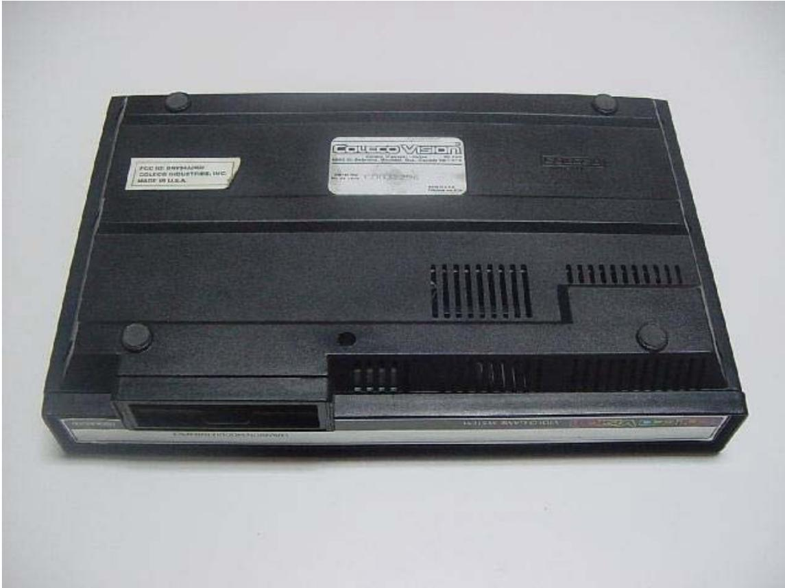
The Colecovision top cover is tricky to remove. After removing the 8 screws you need to pull out on the front edge of the case top where the expansion door is. Continue to work along the front edge until the bottom is free from the top edge as shown below.
