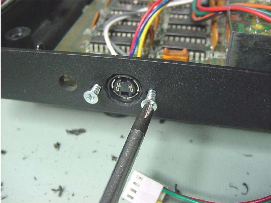
Remove the nut from the black audio jack and insert into the left hole of the case
